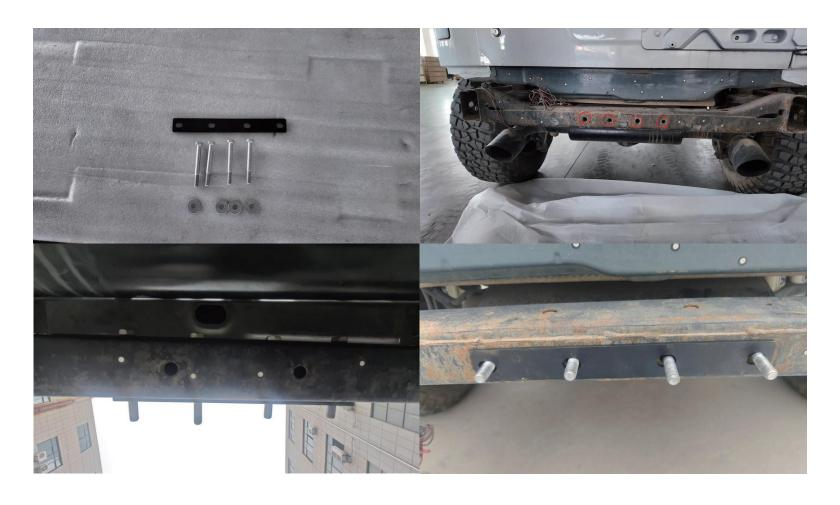
Prepare required parts (①×1, d×4, h×4). As shown in the diagram, insert ①, d, and h in reverse into the red circle markings.
