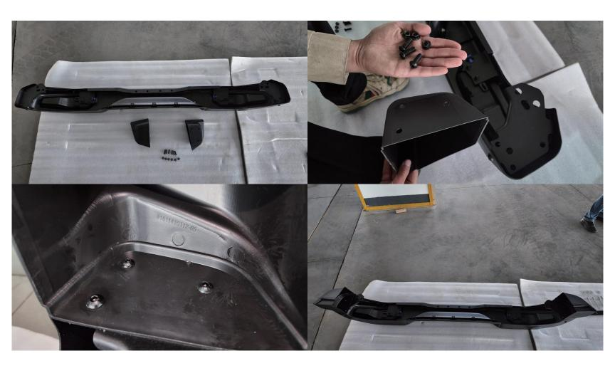
Prepare required parts ( $\textcircled{4}\times2$ , b×6, g×6). As shown in the diagram, use b and g to connect 4 and bumper.
