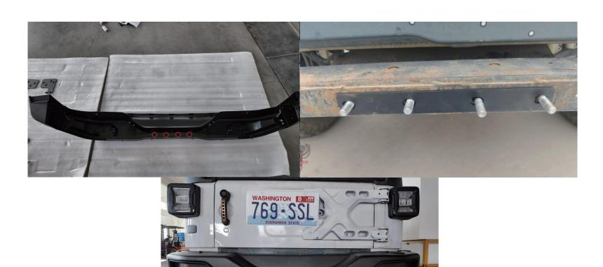
Align the holes circled on the bumper with d, then install onto the vehicle.
