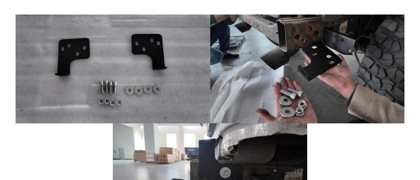
Prepare required parts (③×2, c×4, e×4, h×4). As shown in the diagram, use c, e, h to secure ③ to the red circle markings. (Note: Do not tighten.)
