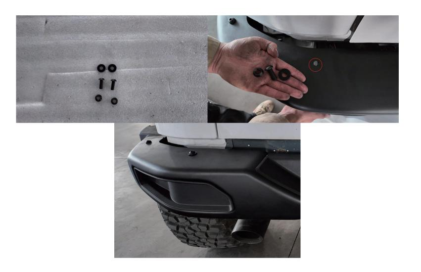
Prepare required parts (a×2, f×2, i×2). As shown in the diagram, use a, f, i to connect the bumper and ③ at the red circle markings.
