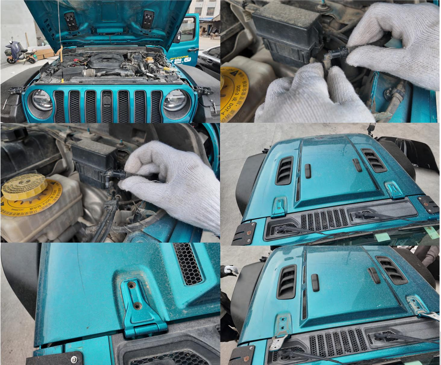
Open the hood, disconnect the washer fluid hose, close the hood, remove the hinge screws, and detach the hood from the vehicle .
