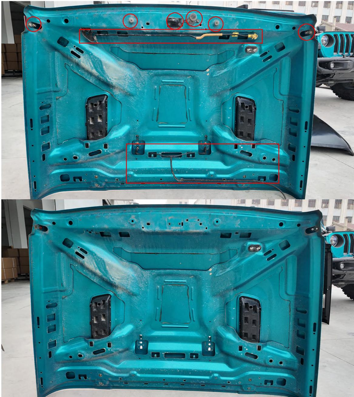
As shown in the diagram, remove all boxed components.
