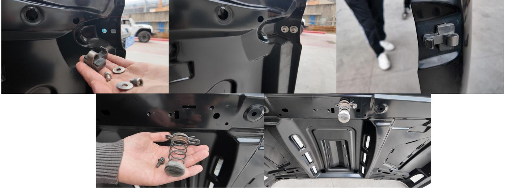
As shown in the diagram, install the original vehicle components onto the new hood.
