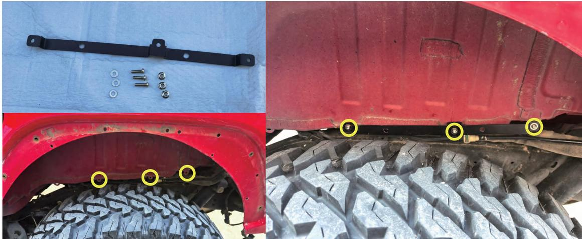
Assemble the necessary components for installing the inner fender liner and position them as shown in the diagram.
