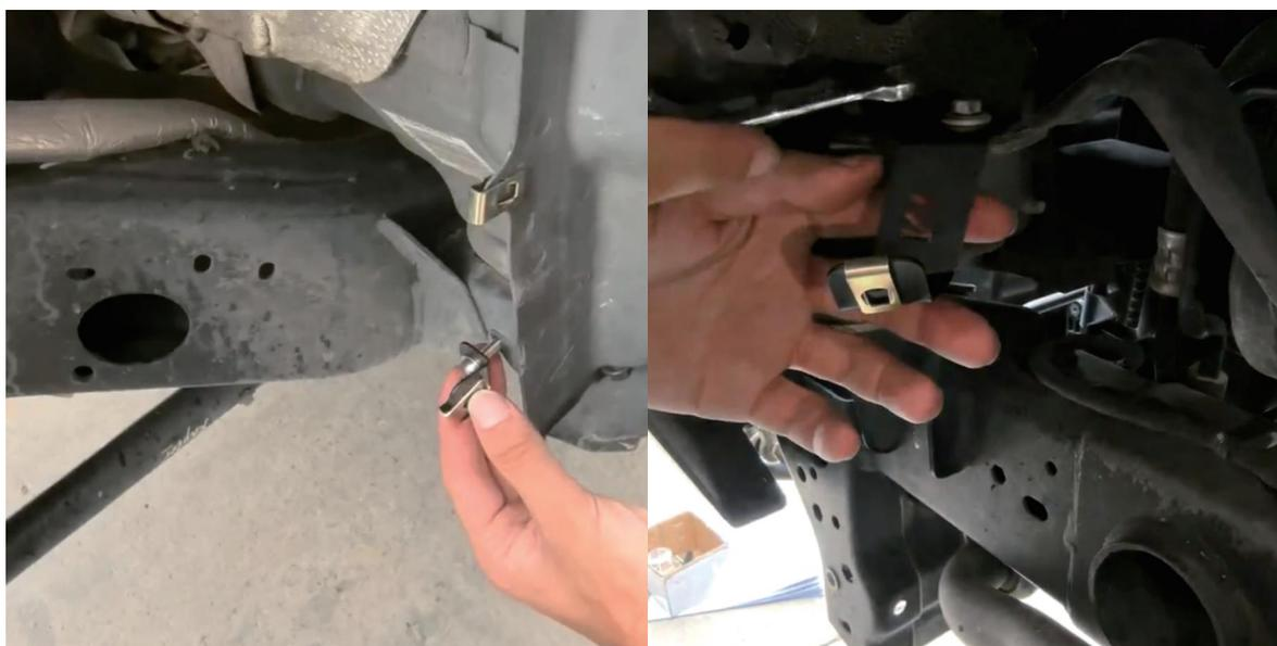
Secure the lower mounting point using the bolts, washers, threaded plate (item no.6). Connected by the clip nut.
