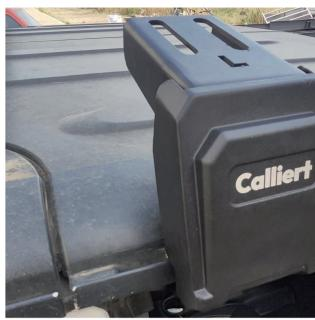
Prepare the required components (E x4). First, loosen the two screws at the bottom of E, then snap E into the rain channel as illustrated.
