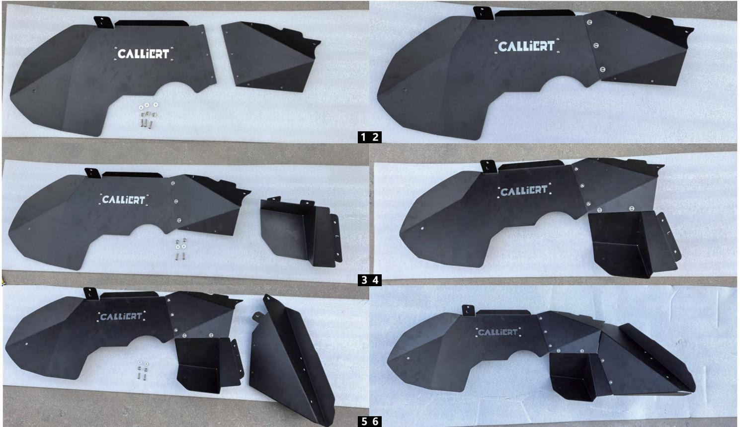
Begin by unpacking all items and inspecting them for damage or missing items. Any concerns, please contact the company you purchased the inner fenders from. Hardware required. Preassemble the front inner fender liner using bolts, washers, nuts. Leave the bolts finger tight, as they will be tightened in a later step.
