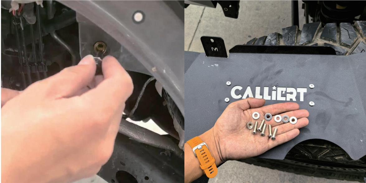
Install the rivet nut into the designed hole.
