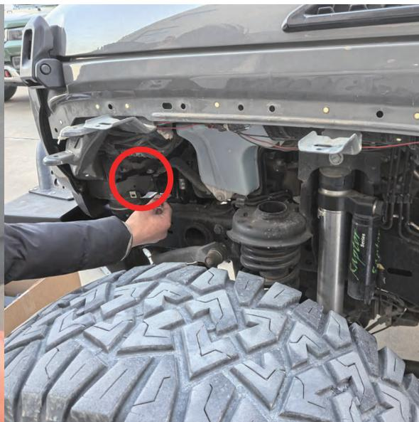
Secure the lower mounting point using the bolts, washers, threaded plate (item no.6). Connected by the clip nut.
