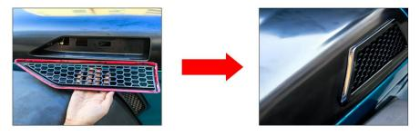
4. Attach the vents to both side of hood by included 3M tape.
