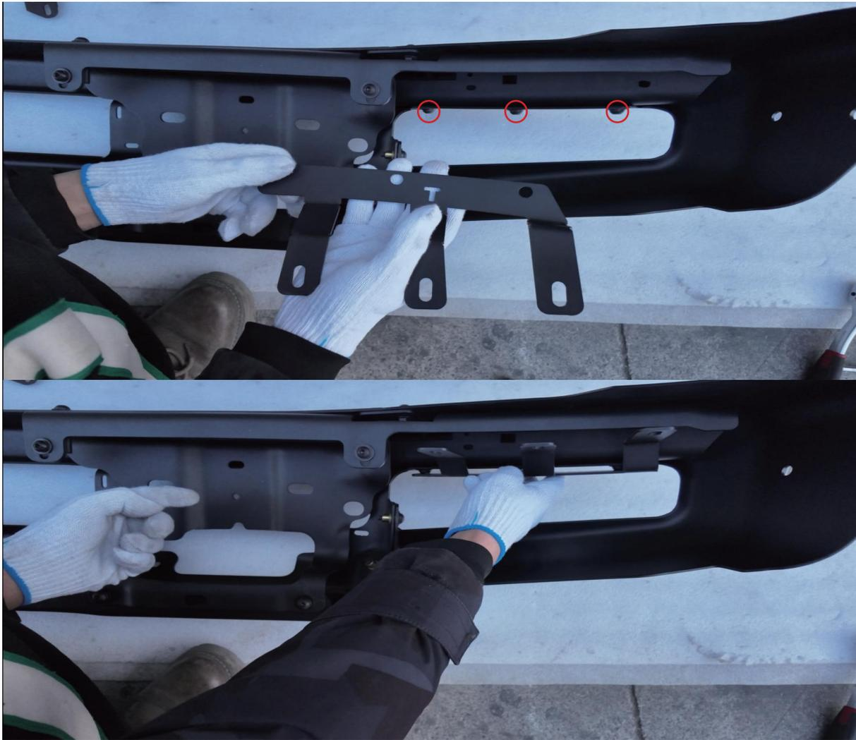
If installing spotlights, as shown in the diagram, remove the screw at red-circled area, then install ⑥ to red-circled mounting hole using the removed screw.
