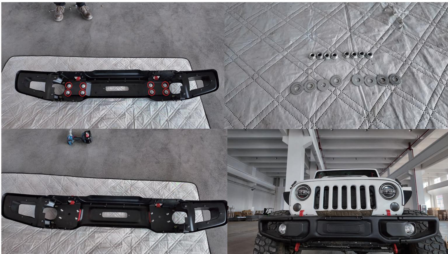
As shown in the diagram, connect the bumper and vehicle beam using screws and washers removed from ⑩.
