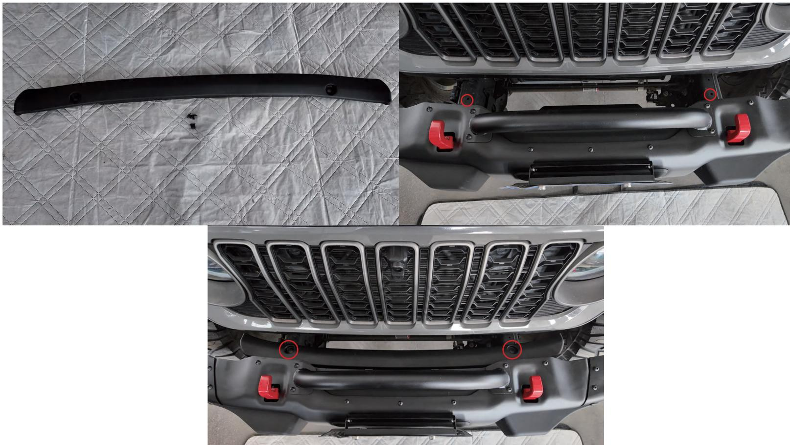
As shown in the diagram, connect (10) to beam at circled holes.
