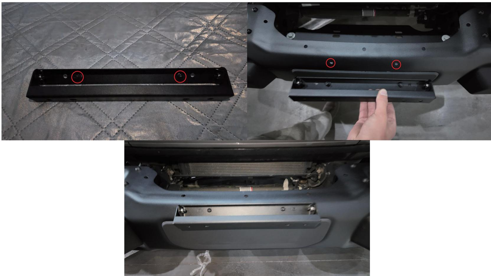
Remove circled screws, then connect ⑧ to bumper using removed screws.
