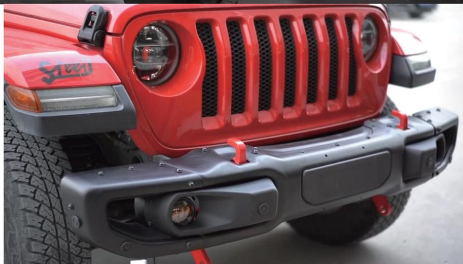
Align bumper screws with circled holes, then secure bumper and beam using removed washers and nuts.
