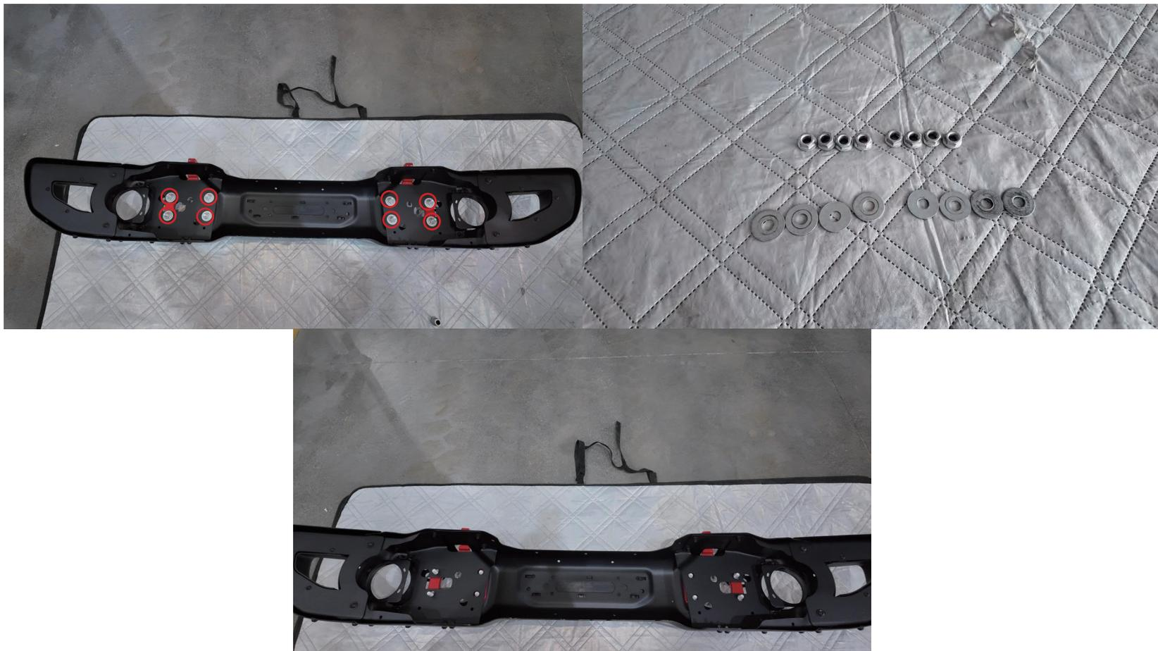
As shown in the diagram, remove circled washers and nuts.
