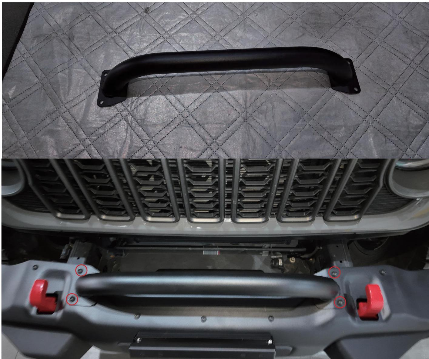
Remove circled screws, then connect ⑨ to bumper using removed screws.
