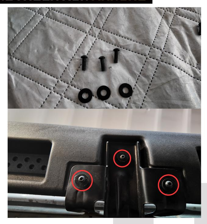
After firmly fixing the brackets, locate the required screws. Connect the brackets and running boards using E and F screws.
