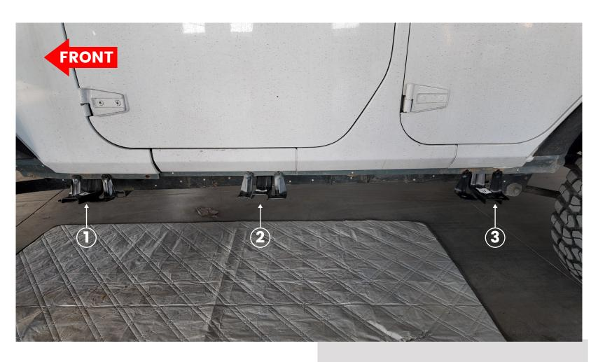
Install the brackets onto the car's side skirts following the numbered sequence.
