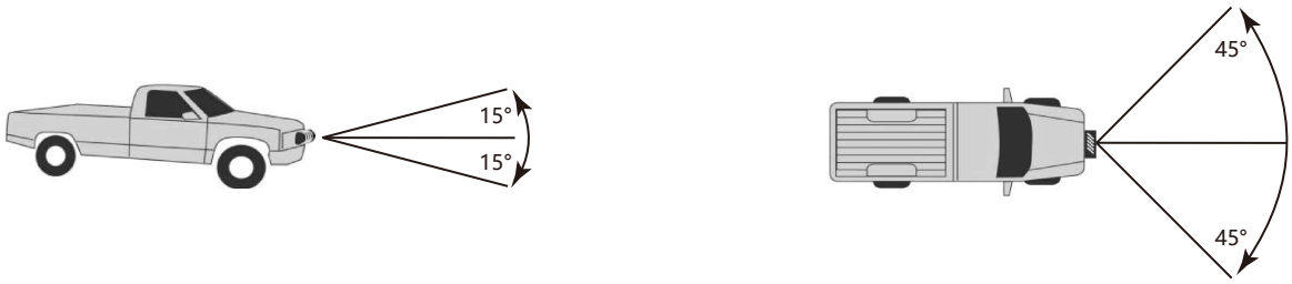
Figure B: Roller Fairlead Maximum Winching Angles
